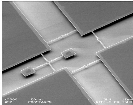
Figure 1: Microfabricated metal heater lines suspended 1.0  $\mu\text{m}$  above the substrate, for thermal property measurements.
