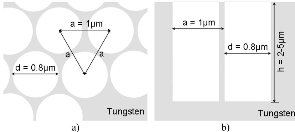
Fig. 3. Dimensions of the selective emitter structure to be produced in tungsten:
