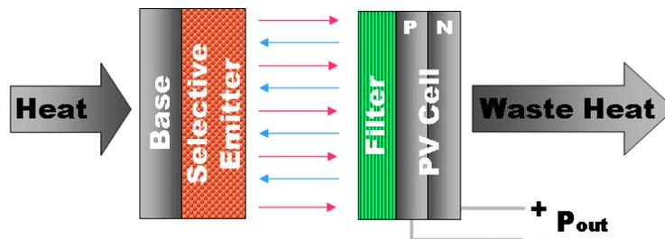
Fig. 1. TPV power conversion system with spectral control components.
