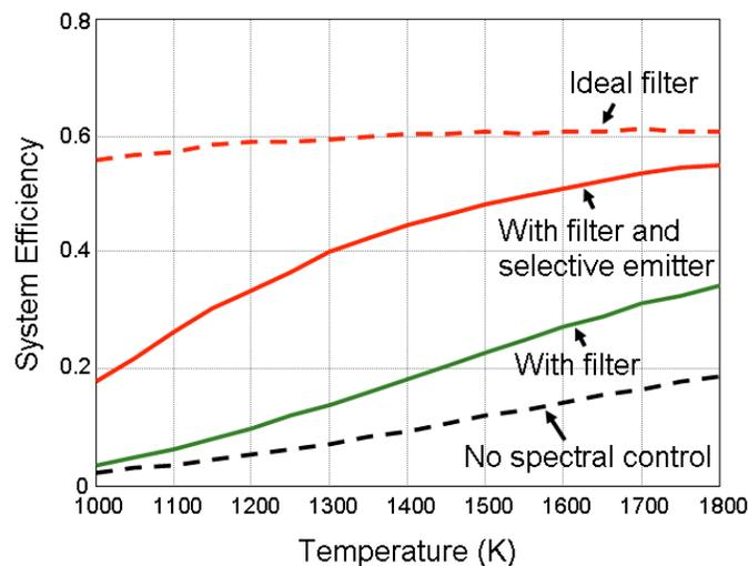
Fig. 2. Efficiencies of TPV systems with various spectral control options.
