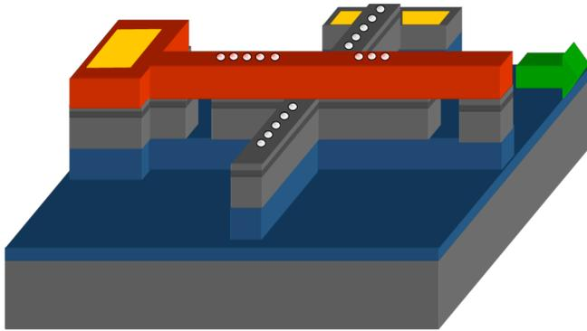
Figure 1: Depiction of the electrically-activated photonic crystal nanocavity laser. The green arrow represents the direction and location of the emitted light.
