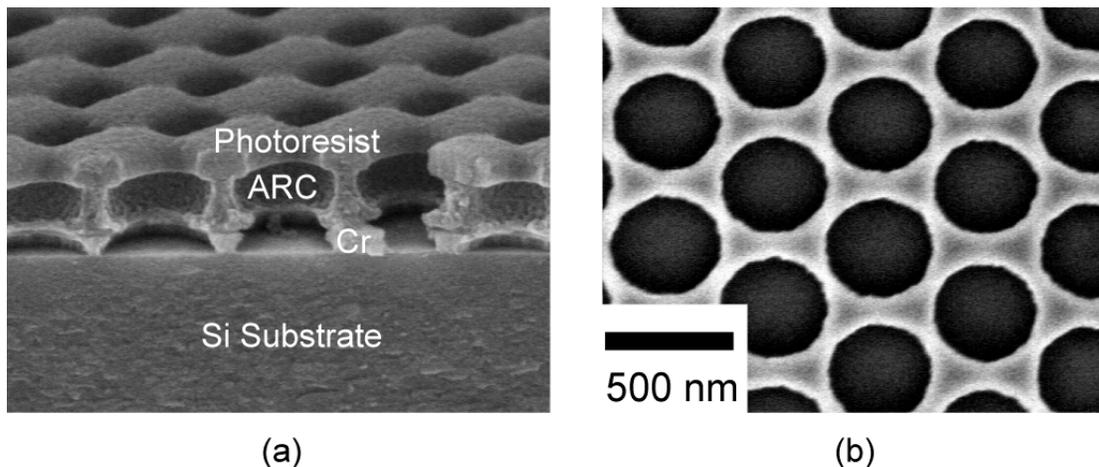
Figure 1. Mechanism and results of the dual-wet-etch process. (a) The photoresist has elliptical holes patterned with IL double exposures  $60^\circ$  apart. An anti-reflective coating layer (ARC) is etched with the same developer as the photoresist. Clear undercuts can be observed. The holes in Cr layer is also defined with a wet etchant (CR-7). (b) The result of the dual wet etch process. The PhC pattern in Cr has almost circular holes.
