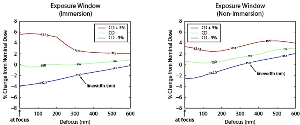
Figure 7: A comparison of the exposure windows for the immersion and non-immersion ZPAL systems. The area between the CD+5% and CD-5% curves defines the exposure window, which is clearly larger for the immersion system.
