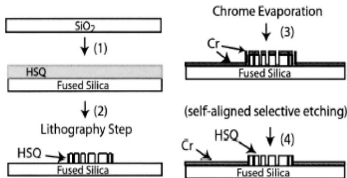
Figure 8: Fabrication of the NIL template.
