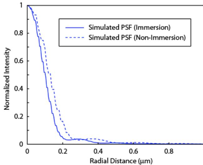
Figure 2: Simulated PSFs of  $NA=0.85$  zone plates operating at  $\lambda=400\text{nm}$  under immersion and non-immersion conditions. The simulations were generated using a Finite-Difference-Time-Domain algorithm.
