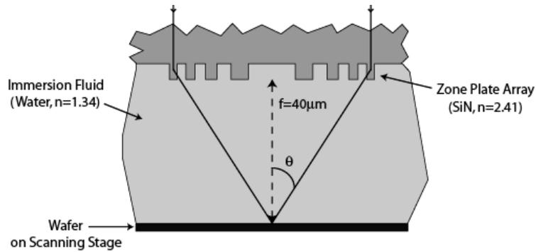
Figure 3: Immersion lithography for ZPAL. We place a droplet of DI water on the substrate, then lower the zone-plate array face down onto the droplet.
