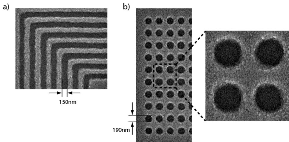
Figure 6: SEMs of (a) nested-L's and (b) arrays of contact holes, demonstrating the performance of the immersion ZPAL system.
