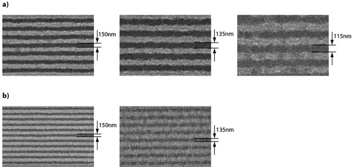
Figure 5: Scanning electron micrographs (SEM's) showing resolution of the immersion and non-immersion ZPAL systems at  $\lambda=400\text{nm}$ . (a) The immersion zone plates reliably print dense lines/spaces down to 115nm. (b) The non-immersion zone plates reliably print dense lines/spaces down to 135nm.
