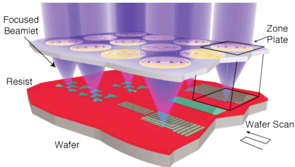
*Figure 1: Schematic of Zone-Plate-Array Lithography (ZPAL). An array of Fresnel zone plates focuses radiation beamlets onto a substrate. The individual beamlets are independently turned on and off by upstream micromechanics as the substrate is scanned under the array. In this way, patterns of arbitrary geometries can be created in a “dot-matrix” fashion.*
