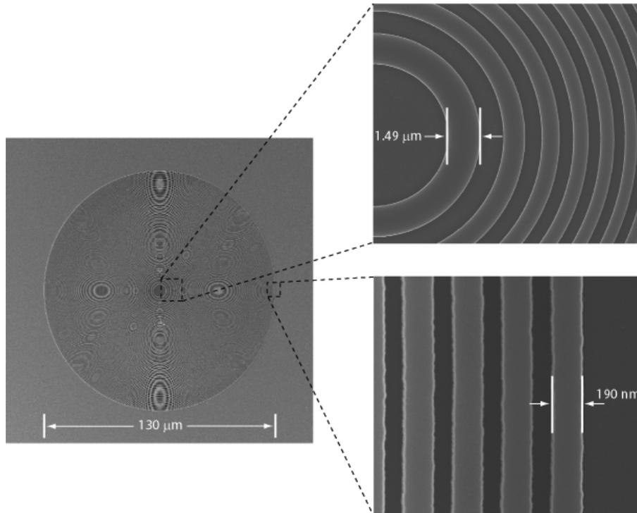
Figure 4: SEMs of an  $\text{NA} = 0.85$  immersion zone plate, designed for  $\lambda = 400\text{nm}$ .
